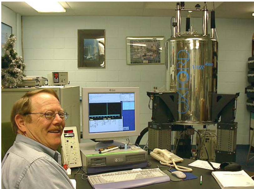
Ron Federspiel hard at work in front of the new Varian ANOVA 500 MHz NMR
