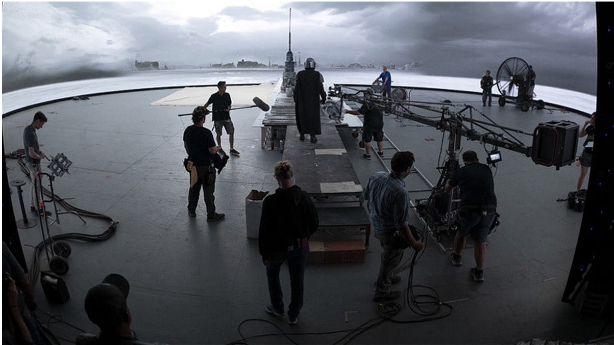
Behind-the-scenes from The Mandalorian (characteristic of modern filmmaking, much of this series is shot on a sound-stage, using a gigantic curved LED screen instead of a green screen to lay in background digital environments)
