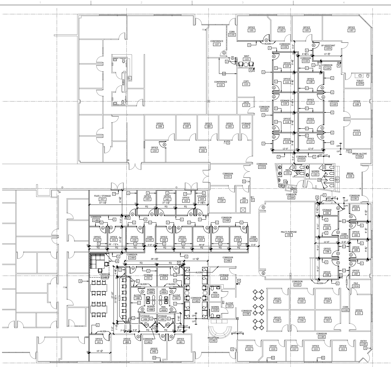
1 PARTIAL FIRST FLOOR CONSTRUCTION PLAN 1/8" = 1'-0"
